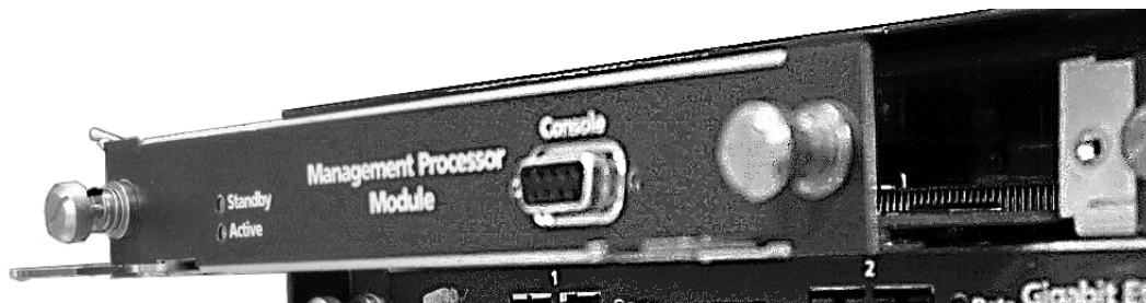
Figure 21 Aligning the Management Processor Module
