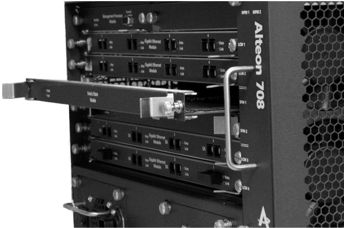
Figure 23 Inserting the Switch Fabric Module
