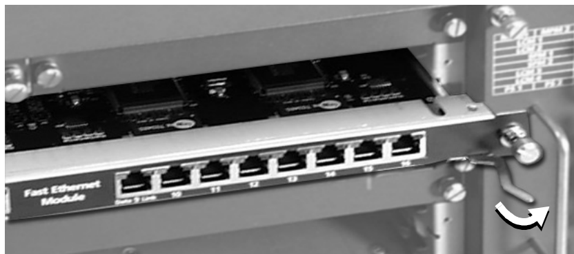
Figure 14 Use the Ejection Levers to Free the Line-Card Module
