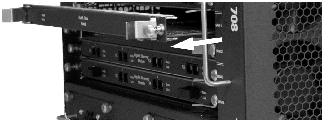
Figure 24 Pulling Out the Switch Fabric Module
